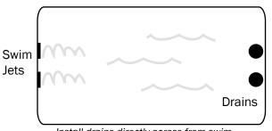
Install drains directly across from swim jets to help pull water from the jets
